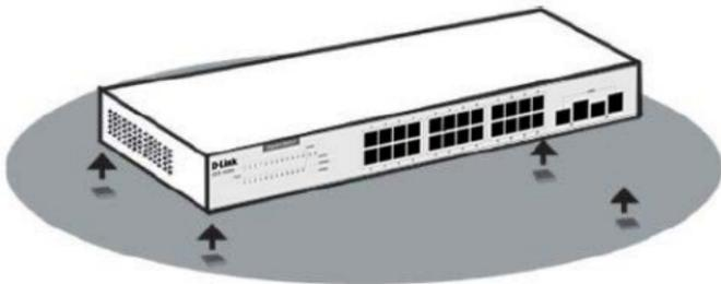
Attach the adhesive rubber pads to the bottom.
