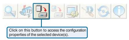
The device configuration window allows you to configure settings but does not actually apply the settings to the device unless you click the **Apply** button. You can also save and load configuration files from this window. When you load a configuration file, you must click **Apply** if you want the settings to be applied to the selected device(s).
