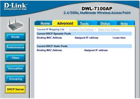
This screen displays information about the current DHCP dynamic and static IP address pools. This information is available when you enable the DHCP function of the DWL-7100AP and assign dynamic and static IP address pools.
