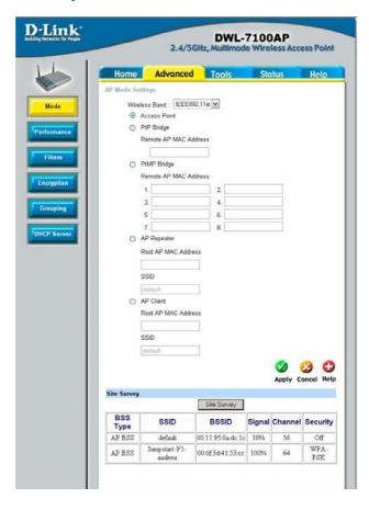
AP Client: will transform any IEEE802.3 Ethernet device (e.g., a computer, printer, etc.) into an 802.11a or 802.11g wireless client when it communicates with another DWL-7100AP that is acting as an AP. Click to enable and enter the MAC address of the DWL-7100AP that is acting as the AP. (Use the Site Survey tool, as described above.)
