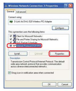
computer has an IP address of 192.168.0.2, the other computers should have IP addresses that are sequential, like 192.168.0.3 and 192.168.0.4. The subnet mask must be the same for all the computers on the network).
