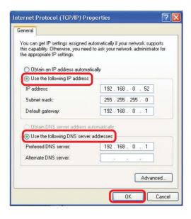
You have completed the assignment of a static IP address. (You do not need to assign a static IP address if you have a DHCP-capable router).
