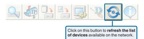
Devices with a checkmark next to them are still available on the network. Devices with an X are no longer available on the network.
