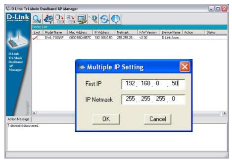
Select the AP that you want to assign an IP address to and click the IP button. Enter the IP address and IP netmask for the selected device and click OK.
