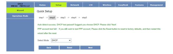
If both DHCP and PPPoE test fails, For SIM card: please verify sim card connectivity (whether the SIM card is active and inserted correctly) For Fibre: please verify that your fibre is active and the cable from the ONT device is plugged into the blue port at the back of the G413K
