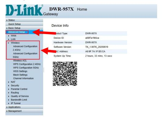
**Step 3:** Look for where it says cannel, currently it should be on auto, if you click on it you will have the option to change it here. For the **2.4Ghz** we recommend using channels **1, 6 or 11** and for the 5Ghz we recommend using channels **36, 40 or 44.**
