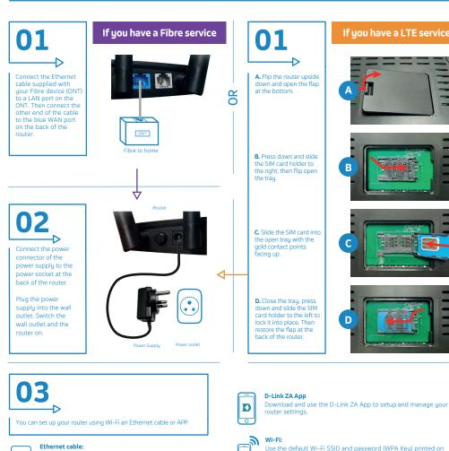
Connect the yellow RJ-45 Ethernet cable to any yellow LAN port at the back of the router and the other end into your PC LAN port.
