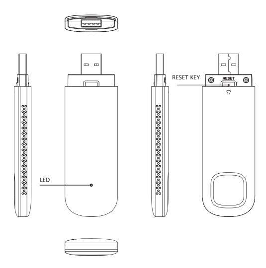
Reset key: press the reset hole with a pen tip or needle for 3-5 seconds to restore the factory settings.
