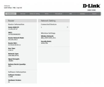
4. You can click the wireless interface to modify the WiFi account and password, modify the MiFi name in "SSID", and change the password in "password";
