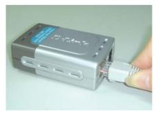
Insert one end of the DC Power Cable that is provided into the Terminal Unit, and the other end into the DC of the Network Device. The Power LED of the Terminal Unit should light up.
