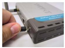
Connect the provided Cat 5 Ethernet cable from the Terminal Unit "LAN OUT" to the RJ-45 LAN port of the Network Device.
