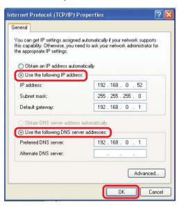
You have completed the assignment of a static IP address. (You do not need to assign a static IP address if you have a DHCP-capable gateway/router.)
