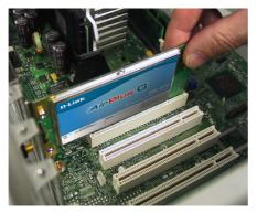
To avoid damage caused by static electricity, make sure to properly ground yourself by first touching a metal part of your computer to discharge any static electricity before working with the DWL-G510 Wireless PCI Adapter.
