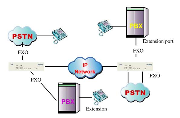
• FXO ports can connect with PSTN Line or Extension Line of PBX
