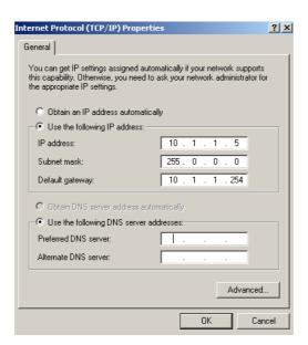
Figure 2.2: Configure the network
