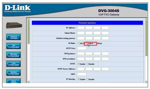
Figure 2.10: Enable the DHCP function
