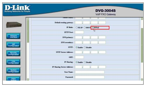
Figure 2.11: Switch to PPPoE function
