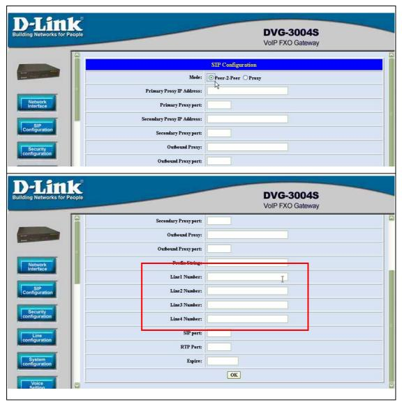
Figure 2.13: Configure the Peer-to-Peer mode
