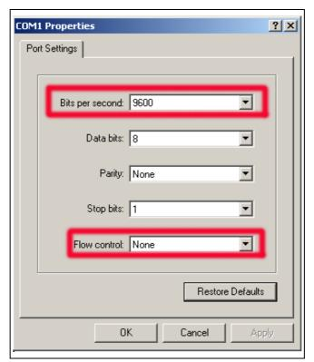
Figure 4.4: Configure the right Bps and control
