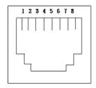
PIN 1, 2: Transmit PIN 3, 6: Receive
