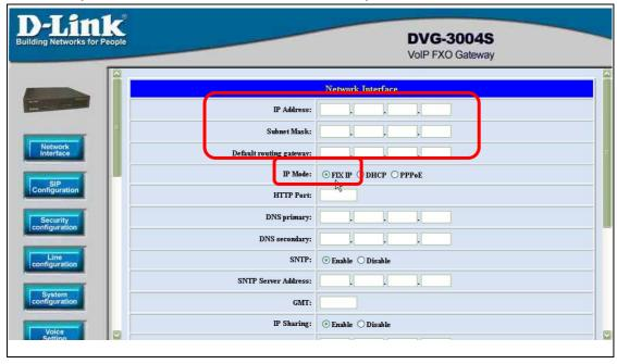
Figure 2.7: Configure the static ip address
