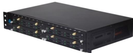
DVG2000-VG-M (Built in 4-1 Antenna Power Divider )
