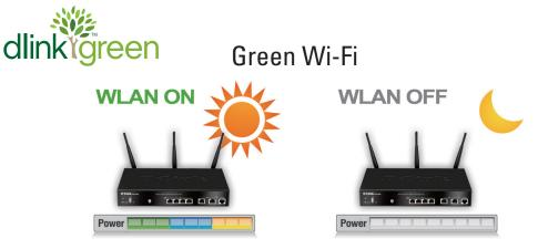
The WLAN Scheduler turns down WLAN during off-peak hours to enhance network security and save power.
