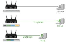
The D-Link Green Ethernet power-saving program can adjust power by detecting link status and cable length.
