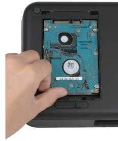
Place the bracket over the hard drive as shown, and secure the hard drive with the included screws. Replace the hard drive cover and slide the drive lock to the locked position.
