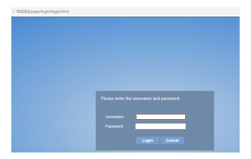
**Note:** If you cannot remember your password or cannot log in, follow the factory reset procedure to restore the router to its default settings. The web interface is used to set up and change settings on the DSL-G2562DG. Follow the steps below to access the web interface and start setting up the DSL-G2562DG.
