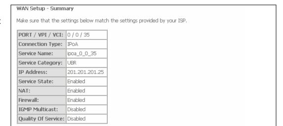
Click "Save/Reboot" to save these settings and reboot router. Click "Back" to make any modifications. NOTE: The configuration process takes about 1 minute to complete and your DSL Router will reboot.
