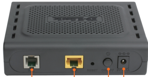
RJ-11 ADSL Port RJ-45 Ethernet LAN Port Power ON/OFF Switch Socket for Power Adapter
