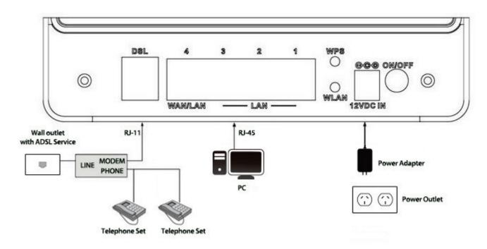
Step 1 Connect the DSL port of the router and the Modem port of the splitter through a telephone cable; connect the phone to the phone port of the splitter through a telephone cable; and connect the Line port of the splitter to the uplink telephone jack on the wall.
