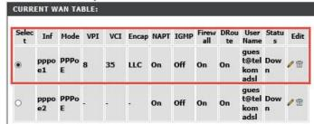
**Step 4**: Scroll up to the Current Configuration, and edit the PPP settings Username and Password with the details provided by the ISP.
