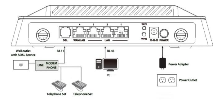
**Step 1** Connect the **DSL** port of the router and the Modem port of the splitter through a telephone cable; connect the phone to the phone port of the splitter through a telephone cable; and connect the Line port of the splitter to the uplink telephone jack on the wall.
