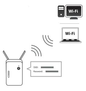
When the LED is blinking amber, connect your PC or laptop to the Wi-Fi name (SSID) printed on the back of the device, or on the included Quick Install Card.
