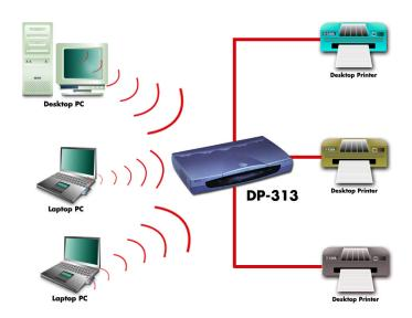
The D-Link DP-313 implements DMA channel support for high-speed simultaneous printing on all three parallel ports.
