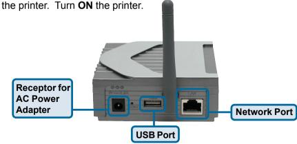
Then, plug one end of the power adapter into the DP-311U and the other end into your electric outlet. The DP-311U will turn on and begin a self-test.
