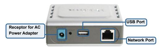
Then, plug one end of the power adapter into the DP-301U and the other end into your electric outlet.
