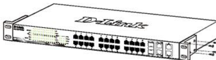
Figure 2.2 – Attach the mounting brackets to the Switch
