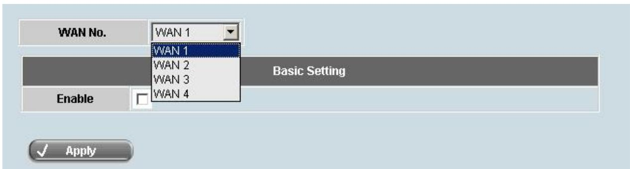
2. In the **[Basic Setting]** table, tick the checkbox next to **“Enable”** to activate the WAN link.
