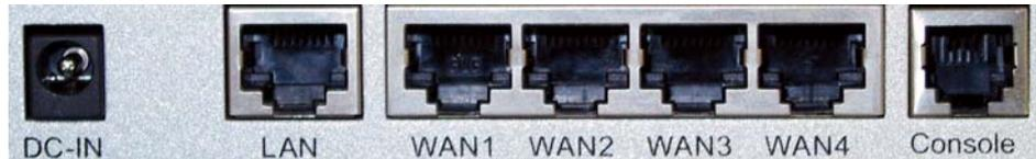
**DC-IN:** The power cord attaches here.
