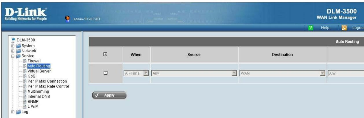
The following configuration is about load balancing with two wan links. In this example, algorithm “Run Robin” is employed to do load balancing with WAN 1 and WAN 2. Click on the **[Service] -> [Auto Routing]** in menu, you could see the **[Auto Routing]** page and the procedure for configuration is listed below:
