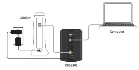
6 After the router has powered up, verify that the Power (green) and internet (orange or green) LEDs are both lit then continue with the *Configuration* After the router has powered up, verify that the Power (green) and Internet section on the other side.
