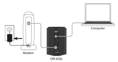
Plug the power adapter into your router and connect to an available power outlet or surge protector. If the Power LED does not light up, press Plug the power adapter into your router and connect to an available the Power button on the back of the router.
