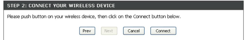
To successfully add a new wireless device, you would have to enter either the PIN information or the button must be pressed within 120 seconds.
