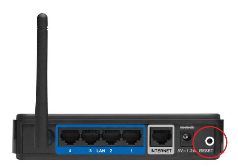
2. Insert a paperclip into the reset pin hole and hold in for 10 seconds. While holding in the reset button, refer to the Power LED, when it turns yellow/orange, release the paperclip holding in the reset button.
