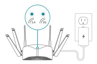
2 / Connect your computer to the Wi-Fi details printed on the Quick Installation Card. Type **http://dlinkrouter.local./** into a web browser. Follow the on-screen instructions to complete the setup.
