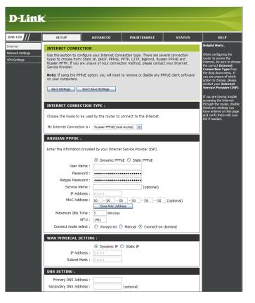
WAN Physical In most cases, select Dynamic PPPoE. Select Static PPPoE if your ISP assigned you the IP address, subnet mask, gateway, Setting: and DNS server addresses.
