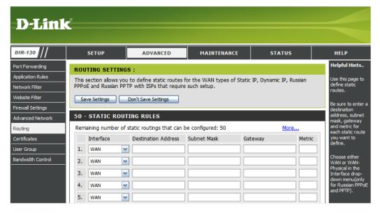
\*PPTP, L2TP, Russian PPPoE, and Russian PPTP Internet configurations and the WAN\_Physical parameter referenced in this section does not apply in North America.
