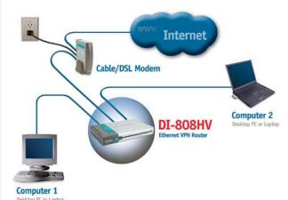
With the DI-808HV, you can share Internet access in your home or office. Connect up to eight computers and an external analog dial-up modem using its available COM port.
