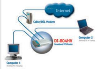
With the DI-804HV you can share Internet access in your home or office. Connect up to four computers and an external analog dial-up modem using its available com port.
