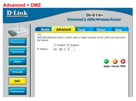
If you have a client PC that cannot run Internet applications properly from behind the DI-614+, then you can set the client up to unrestricted Internet access. It allows a computer to be exposed to the Internet. This feature is useful for gaming purposes. Enter the IP address of the internal computer that will be the DMZ host. Adding a client to the DMZ (Demilitarized Zone) may expose your local network to a variety of security risks, so only use this option as a last resort.
