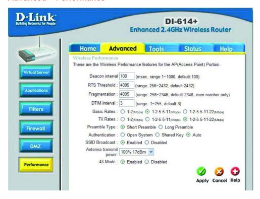
Beacon Interval- Beacons are packets sent by an Access Point to synchronize a wireless network. Specify a value. **100** is the default setting and is recommended.
