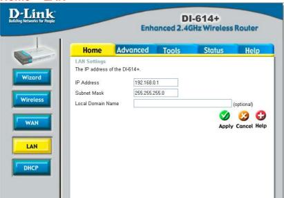
LAN is short for Local Area Network. This is considered your internal network. These are the IP settings of the LAN interface for the DI-614+. These settings may be referred to as Private settings. You may change the LAN IP address if needed. The LAN IP address is private to your internal network and cannot be seen on the Internet.
