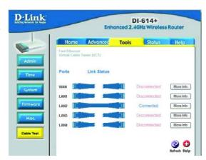
Ports - The Ethernet port names associated to the physical ports.
