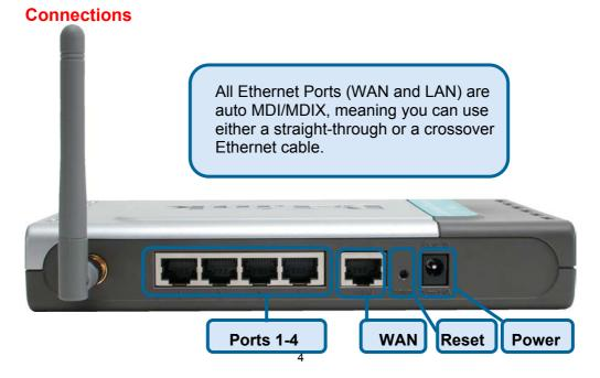
**Reset:** Used to restore the DI-614+ to the factory default settings
