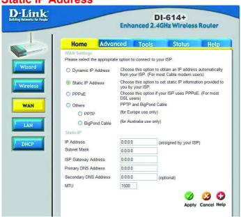
Choose Static IP Address if all WAN IP information is provided to you by your ISP. You will need to enter in the IP address, subnet mask, gateway address, and DNS address(es) provided to you by your ISP. Each IP address entered in the fields must be in the appropriate IP form, which are four IP octets separated by a dot (x.x.x.x). The Router will not accept the IP address if it is not in this format.
