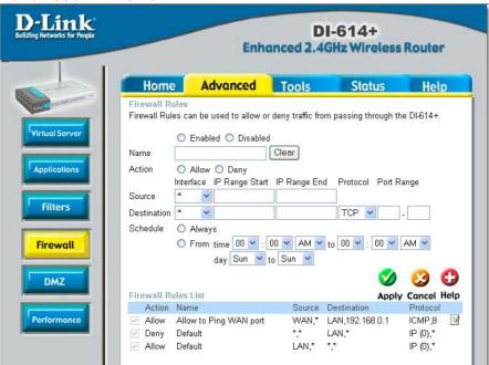
Firewall Rules is an advance feature used to deny or allow traffic from passing through the Broadband Router. It works in the same way as IP Filters with additional settings. You can create more detailed access rules for
