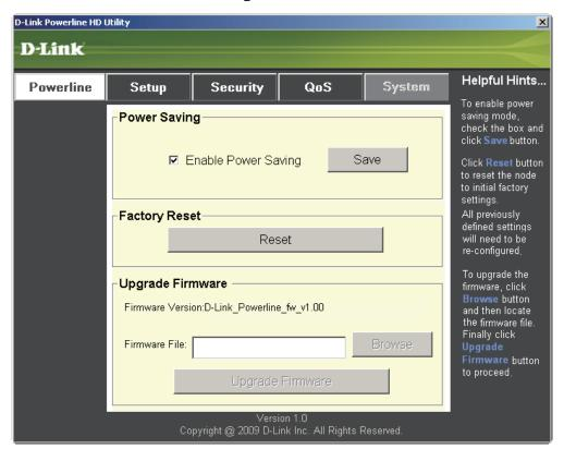
With the power saving mode enabled and the ethernet link activity being down for 15 minutes, the DHP-312 will automatically go into stand-by mode. When the master unit is in stand-by mode, the throughput LED will blink red intermittently.
