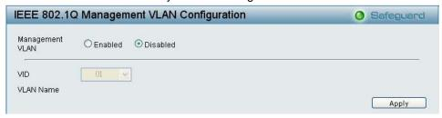
Figure 60 - Configuration > 802.1Q Management VLAN
