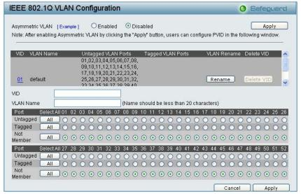
Figure 53 - Configuration > 802.1Q VLAN > Add VID
