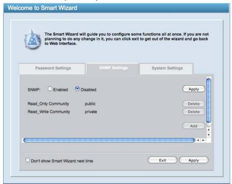
Figure 28 - Configure SNMP in Smart Wizard
