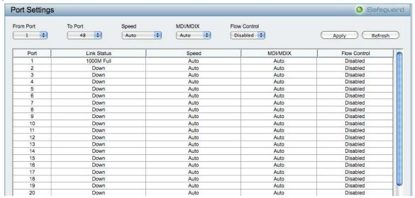
Figure 47 – System > Port Setting
