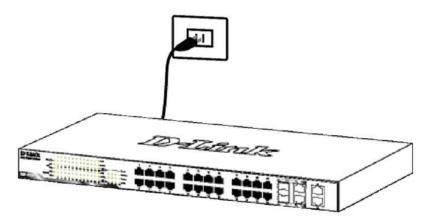
Figure 10 -Plugging the switch into an outlet
