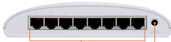
10/100/1000 ETHERNET PORTS Connect computers and devices
