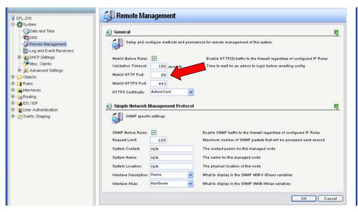
You can also change the validation timeout to 180 sec. That will mean that the firewall will wait for your login for 180 sec before reverting new settings to previous state.
