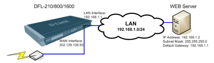
**Step 1.** Log into the Firewall by opening Internet Explorer and typing the LAN address of the Firewall. In our example we are using 192.168.0.1. Enter Username and Password which you specified during the initial setup of the Firewall.
