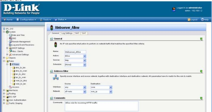
**Step 9.** Rearrange the IP rules so the "Webserver\_SAT" rule is on top, followed by "Webserver\_NAT" and "Webserver\_Allow". To do that right-click on the rule and select "Move Up" or "Move to Top".
