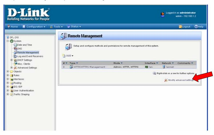
Set WebUI HTTP Port to a different value (e.g. 88). Note that after applying this setting you will need to log into the firewall via new port number: <a href="http://192.168.1.1:88">http://192.168.1.1:88</a>
