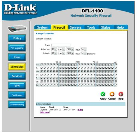
organization may only want the firewall to allow the internal network users to access the Internet during work hours. Therefore, one may create a schedule to allow the firewall to allow traffic Monday-Friday, 8AM-5PM only. During the non-work hours, the firewall will not allow Internet access.
