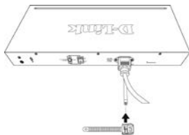
Slide the Retainer through the Tie Wrap
