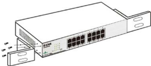
Attaching the mounting brackets to the Switch
