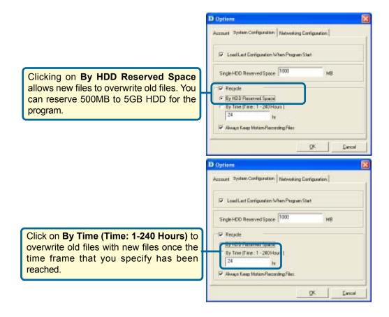
Note: Selecting the **Recycle** option will disable the **Recording File Path Settings** in the **Recording** menu. It is recommended to specify the **Recording File Path Settings** for each camera before selecting the **Recycle** option.
