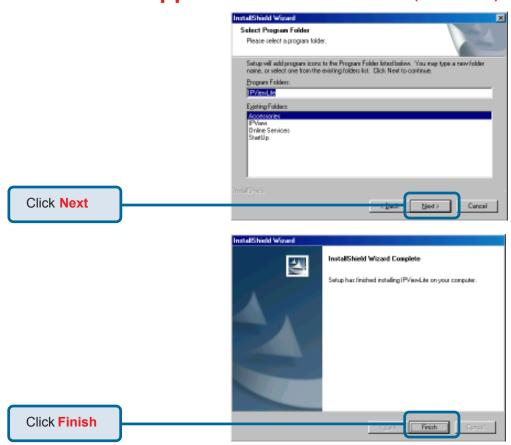
After successfully installing the IPView Lite, the application program for the DCS-900 is automatically installed to \Programs\IPView Directory.
