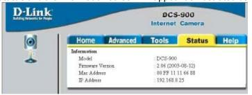
The Information table provides detailed information about the DCS-900 such as the Model Name, Firmware Version, Mac Address, and IP Address.
