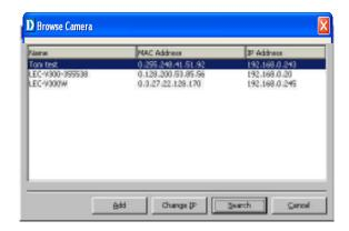
Highlight the camera you wish to add and click on **Add**. The **Add Camera** dialog box will appear once again with the IP Address entered. Click on **Add**. The camera will be automatically added into the IPView Lite list view format.
