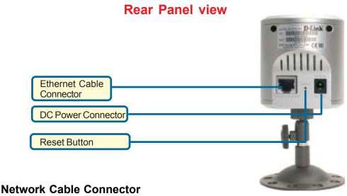
The DCS-900 features an RJ-45 connector for connections to 10Base-T Ethernet cabling or 100Base-TX Fast Ethernet cabling (which should be Category 5 UTP twisted-pair cable). The port supports the NWay protocol, allowing the DCS-900 to automatically detect or negotiate the transmission speed of the network.
