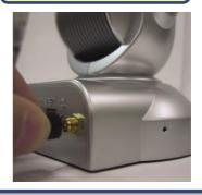
Attach the A/V cable to the A/V out connector if you wish to connect the **DCS-6620G** to your TV set.
