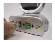
It is required that an Ethernet cable is used during initial setup. Once your wireless configuration is set, you may disconnect the Ethernet cable and reboot your camera to connect to your wireless network.
