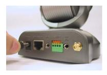
When you have a proper connection, the **LED** (Light Emitting Diode) on the front of the camera will change from red to green. The light may blink on and off and your computer may show an intermittant loss of connectivity, this is normal until you have configured vour camera.
