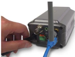
**Note:** When you have a proper connection, the LED will turn from red to green. The light may cycle on and off and your computer may show an intermittent loss of connectivity, this is normal until you have configured your Internet Camera.
