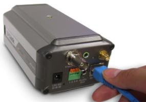
**Note:** It is required that an Ethernet cable is used during initial setup. Once your wireless configuration is set, you may disconnect the Ethernet cable and begin communicating wirelessly with your DCS-3420.
