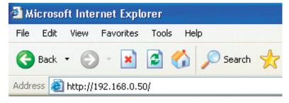
Note: If you have changed the default IP address assigned to the DAP-1160, make sure to enter the correct IP address.
