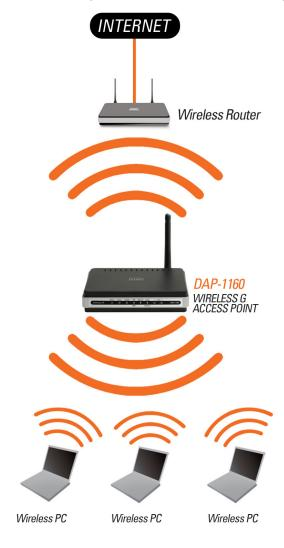
**Extending the Wireless Coverage of a Wireless Router Using the DAP-1160**
